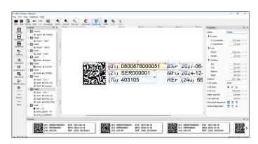
MCX UniDraw is used to design and set up print jobs for HSAJET® MCX printers. It is a user-friendly and flexible software offering all features needed to create print jobs for coding and marking applications.
