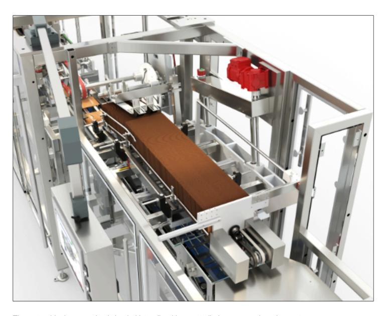
The carton blanks magazine is loaded laterally with a controlled pressure advancing system. Carton blanks pick-up by means of suction cups with a Venturi vacuum system.
