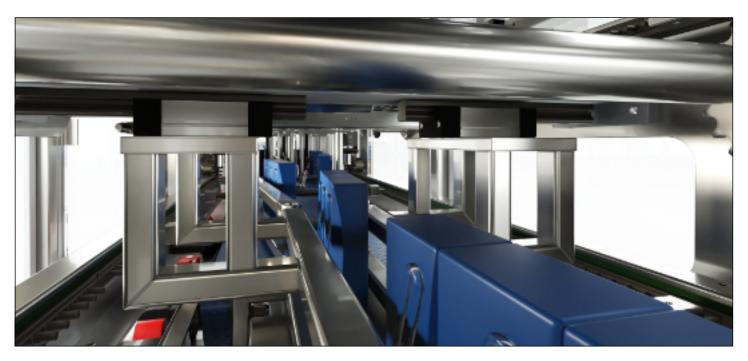
Products arriving on the in-feed conveyor are arranged and laned by means of special parallel belts at machine's entry, distributed into one or two rows and grouped according to the required formats to be packed.
