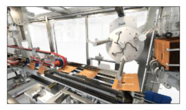
At the same time, the flat carton blanks previously fed from the automatic carton blank magazine by means of a special rotary feeder designed with 3 alternating arms complete with suction cups, places the blank
