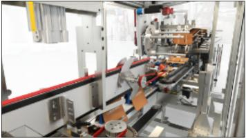
directly above the products in the collation station. The product positioning is synchronised with the blank feeding and the blank is then wrapped around the collation and glued on the base.
