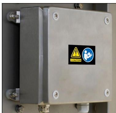
FIM enclosure box mounted onto the conveyor
