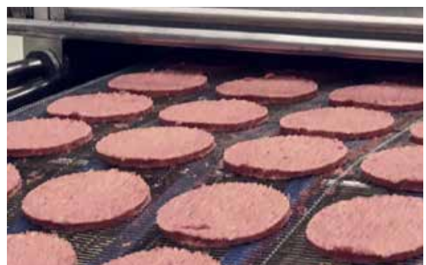
Burger patties approaching the X39 x-ray inspection system
