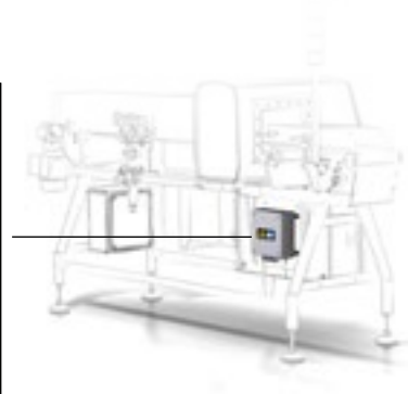
FIM enclosure box mounted onto the conveyor
